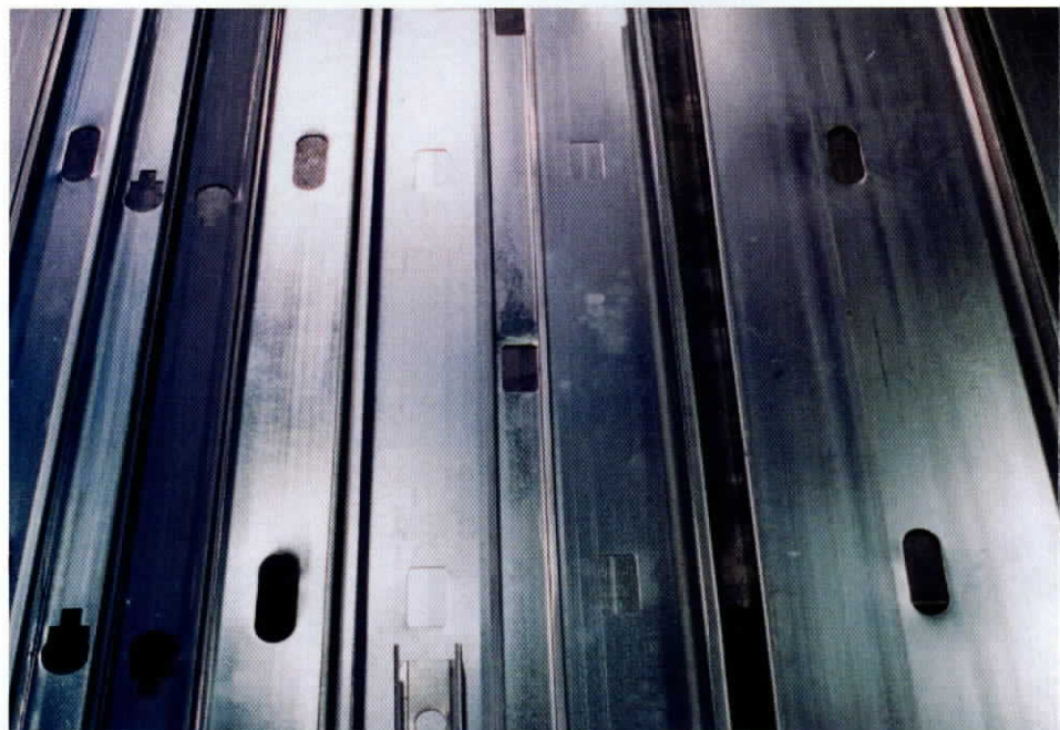
A sample of the structural shapes produced by Hill Engineering's B&K cam-action rotary punch and shear. DC servo drives operated by a programmable logic controller vary hole spacing and part length on the fly. Photographs by the author.
