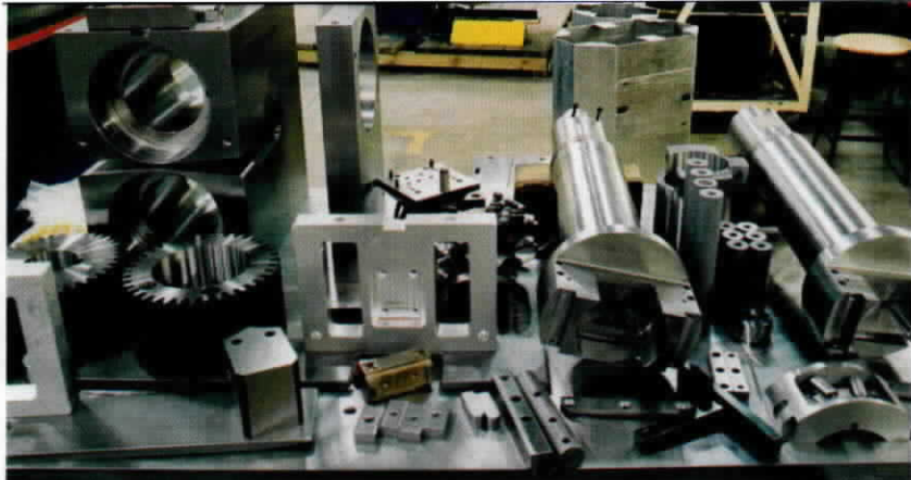
More than meets the eye: A disassembled B&K rotary punch demonstrates the complexity of the cam action that accommodates thicker metal than conventional fixed-punch units.
